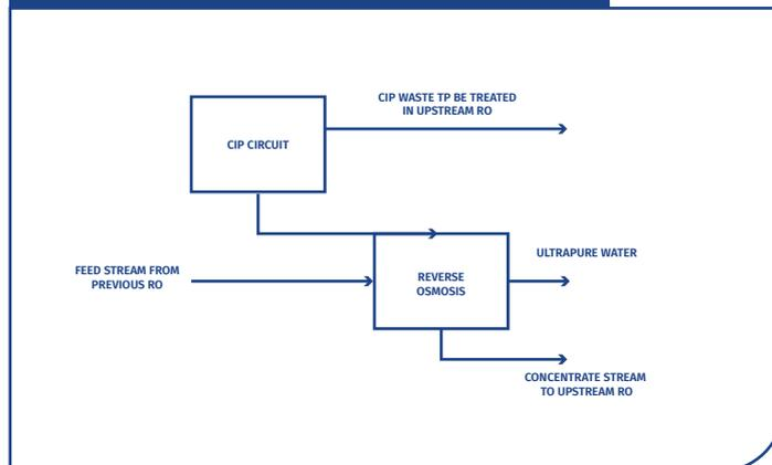
RO Plant 3 is the final RO unit, fed from the nickel (RO Plant 1) and sodium reverse osmosis permeate streams (RO Plant 2), to produce ultra-pure process water for re-use in the plant with no pre-treatment. RO Plant 3 optimises water usage, by producing water to recycle.
