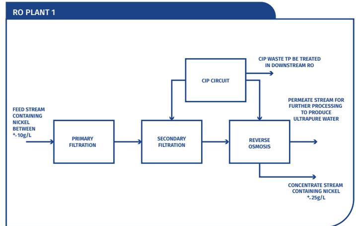
Purification Plant. The nickel is upgraded into the concentrate stream, which is important for the minimisation of downstream dilution of the main nickel concentrate stream feeding the crystalliser.
