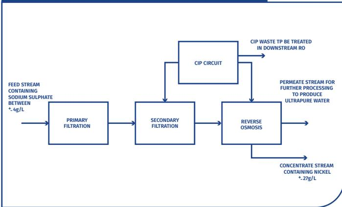
filtration and secondary filtration followed by reverse osmosis. The major role of the sodium RO circuit is to concentrate the sodium as much as possible, reducing the volume of concentrate to be disposed of.
