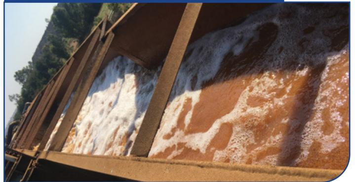
rate achieved is as high as 25,4 m/hr. Inlet total suspended solids is typically 3000 ppm, and the overflow total suspended solids ranges between 5-20 ppm.
